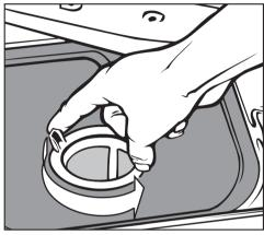
■ To unscrew the micro-fine filter, grasp the two tabs and turn counterclockwise twice.
